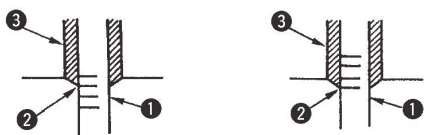
Relation between needle and engraved lines
